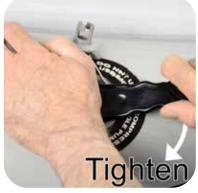
Press on center of valve tool with free hand to keep from breaking the teeth off the tool. If loosening a very tight valve, an extension tube might be needed.
