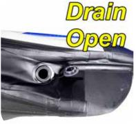
Unscrew the drain cover when draining is needed. Tip the kayak up as necessary for water to flow through the drains.
