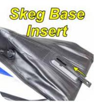
Slide the Skeg Base Insert into base. The insert will help prevent skeg base from becoming warped while the boat is stowed.
