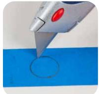
Pro Tip: Trace the outline of the penny on masking tape and cut with a utility knife. Apply tape to the boat instead of tracing on the boat.
