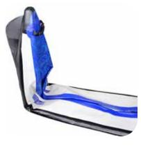
At the front of the boat, make a crease in the middle of the SeaEagle.com logo and fold it back and push the bow off center to the side opposite of the back fold.
