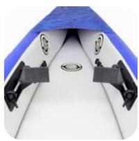
Lock the bar in place by rotating the handle down into the locking hook.
