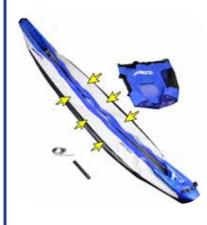
**473rl Folding**Open valves to let air out and push sides inward over the floor.
